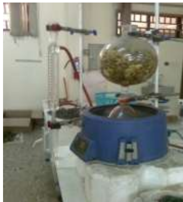
Figure 2. Steam distillation of the Lime peel in a Clevenger-type apparatus to produce the essential oils
